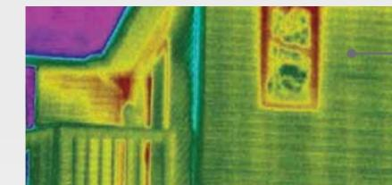
Studs create a thermal bridge for heat to escape in winter and enter your home in summer. Because studs can represent up to 25 percent of the wall surface, it's like having an entire wall without significant insulation.
